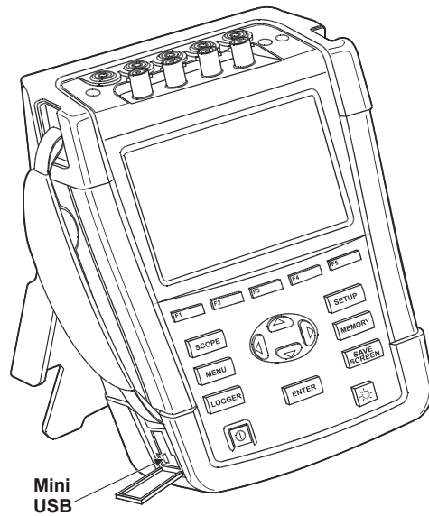
Figure 25-1. Location of USB interface connector
